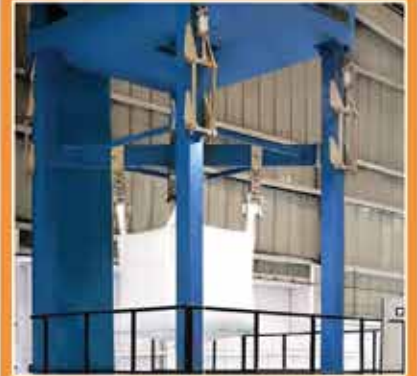
Load Testing machine
